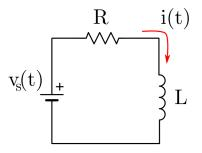
**Solution:** We want to find the equation for output i(t). Start by applying KVL
